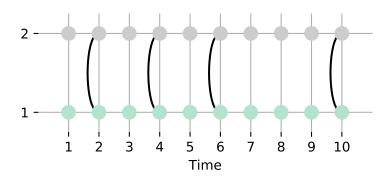
Calculating the inter-contact times of these edges becomes: 2,2,4 between nodes 0 and 1.
